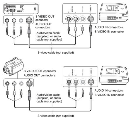
For a camcorder with an A/V OUT connector, you can use an AV cable with S-video to connect to the DVDirect.
